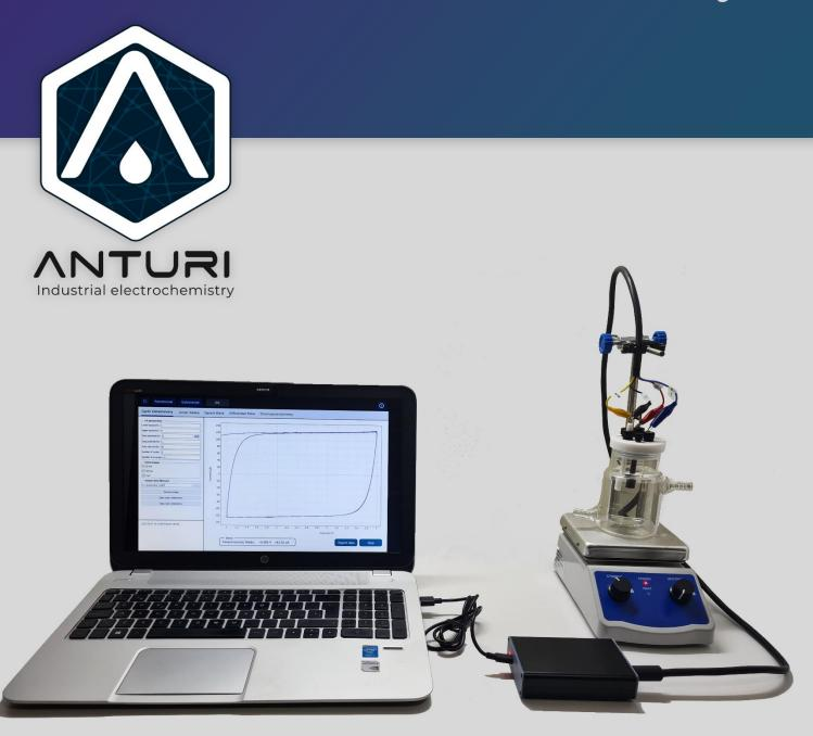
We offer portable **Potentiostat/Galvanostat (PGSTAT)** devices. Small and extremely powerful tools designed to provide a wide range of measurements and high resolution, keeping very low prices compared with the similar devices, with the best-known price-quality of the market.
